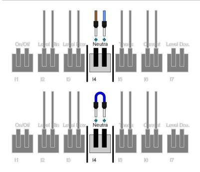
If the input is activated while a contact is closed, the automatic scrubbing liquid change is released. Otherwise the fume scrubber recognises that the neutralisation unit cannot absorb liquid and will not release the scrubbing liquid.
