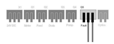
Contact open when fault-free, closed in the event of faults
