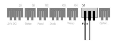
Contact closed when fault-free, open in the event of faults
