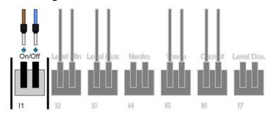
If the input is activated while a contact is closed, the device will switch on. Otherwise the device switches off. The contact can be connected with the ventilation unit installed by the customer or with the frequency converter controlling the fan.
