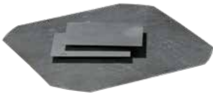
Test plate made of silicon nitride
