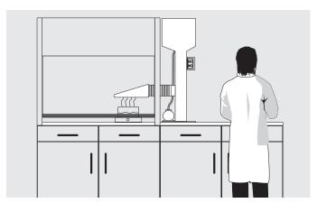
The fume scrubber C20 is flexible in its installation. Besides an installation on benches or on the floor it can be placed where the installation of a fixed scrubber is not possible due to restrictions of space. Please note that the unit must not be installed inside a fume cupboard.
